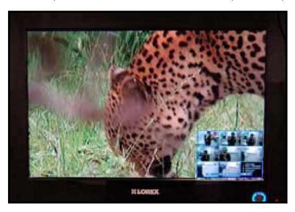
If you press the PIP button on your remote control, you can view your DVR in a Picture In Picture. This provides you with the ability to view images from your cameras while watching a movie.
